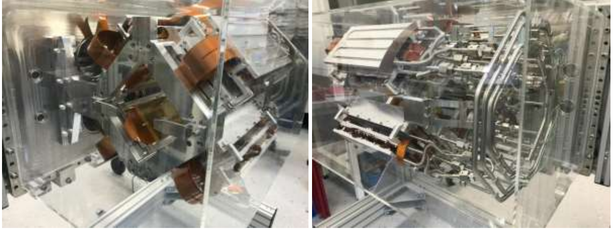
Figure 2: Pictures of the fully assembled PAX detector with four complete quadrants [3].
